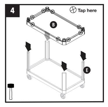
Lower middle tray (B) and insert on top of corner posts (E). First, push down all four corners evenly by hand. Then, evenly tap with mallet on locations indicated until fully seated and secure.
