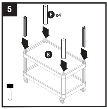
Lower each corner post (E) onto tray (B). For proper alignment, first push down by hand. Then, evenly tap each post with mallet until fully seated and secure.
