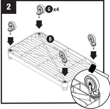
Insert Caster Socket (F) into each corner in bottom tray (B). Evenly tap each caster socket with mallet until fully seated and secure.
